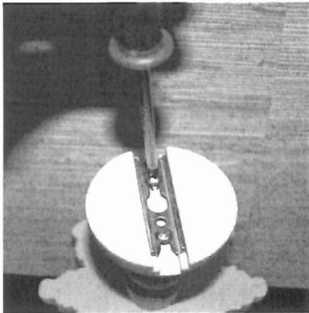
Un screw 1/4 turn and remove brass mounting plate
