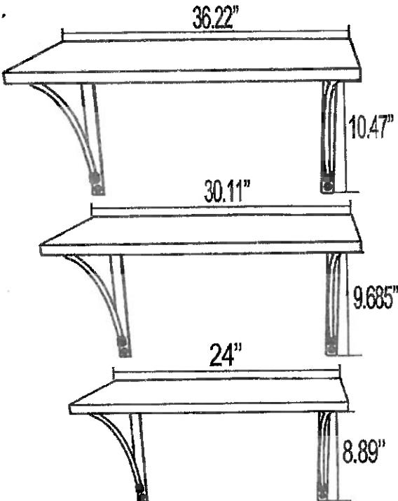
1. Measure and mark the distance on the wall , attach side brackets (B) to the wall by screws.
