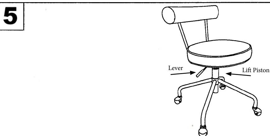
To activate the Lift Piston (Part D), apply weight by sitting in the chair; raise the seat using the lever.
