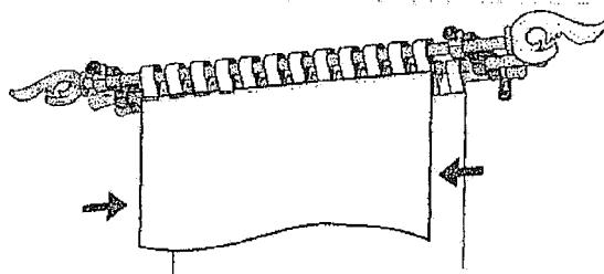
**7** Secure the rod in place by tightening screw.
