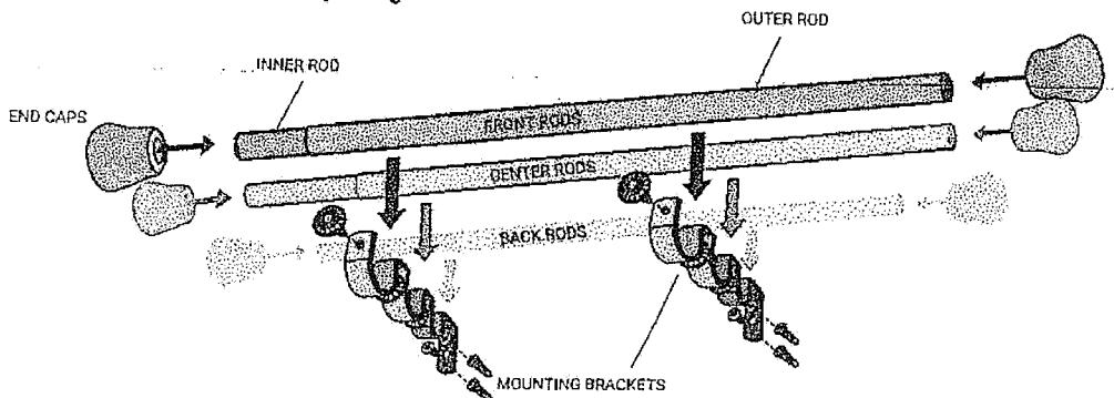
**1** Place the brackets against the wall and mark the screw placements with a pencil. Make sure the marks are level.
